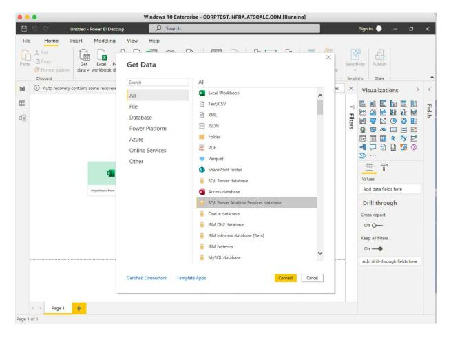
In this image, you can see how the Power BI users can leverage the built-in SQL Server Analysis Services (SSAS) connector. This means that there is no need to install custom client-side drivers to access AtScale models.
